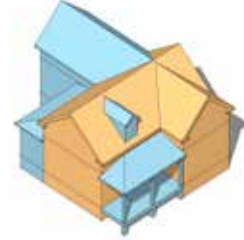
One and one-half-story L-shape with porch tucked into the inside corner
