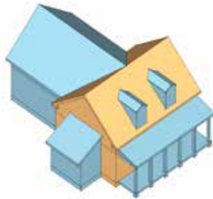
One and one-half-story side gable with full front porch
