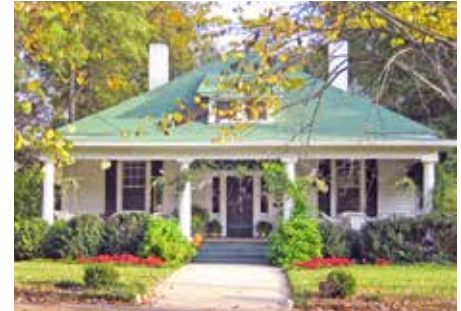
One-story narrow hip massing with full-front porch integrated into the main body roof form
